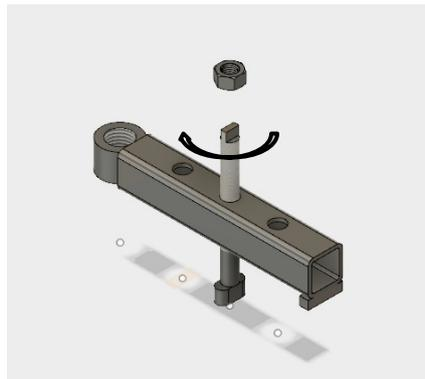
2. Insert and screw pressure bolt into threaded load bar nut.
